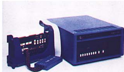
ICE™-80, the first in-circuit emulator, shown with one of Intel's microcomputer development systems. Introduced in 1975, ICE modules could be substituted for the microprocessor components that were actually used in a customer's system, providing a valuable tool for developing and debugging microprocessor-based systems.
