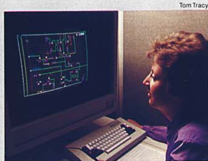
Intel was one of the first companies to use computer-aided design (CAD), now standard throughout the industry. Much of the circuit design and fabrication is now performed on computer-aided workstations—sophisticated computer systems with color display screens. CAD has replaced the painstaking manual operations performed in early circuit design, enabling the development of extremely complex circuits that would be impossible otherwise.
