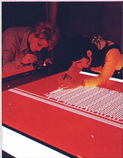
In Intel's early days, each layer of an integrated circuit design was drawn by hand, then transferred onto rubylith. Operators such as the two women pictured here worked at light tables cutting each vector onto the red cellophane-like sheets. The rubylith was then photostepped to the correct size and a mask was made.
